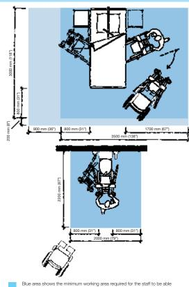
Blue area shows the minimum working area required for the staff to be able to use the mechanical aids in an ergonomic way from one side.
